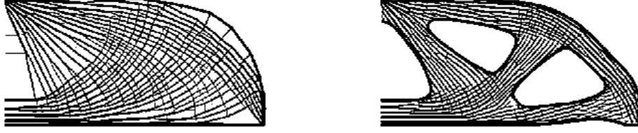
Figure 4: Left: The shell-infill composite obtained with the global volume constraint Eq. 29. Multiple large void parts appear in the base region, counteracting the intent to have distributed infill. Right: Composite obtained with the updated global volume constraint Eq. 31. Infill spreads over the entire base, making a clearly distinguishable shell-infill composite. The compliance is 98.2 (left) and 108.0 (right).
