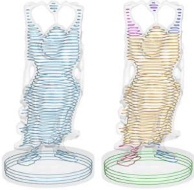
Fig. 7. Contours on the Buddha model (left) are clustered into seven different groups, which are displayed in different colors (right). Contours in each group are connected by strip triangulation to generate an interior surface with simple topology (i.e., genus zero).
