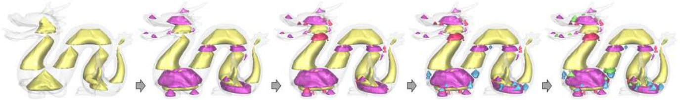
Fig. 12. The volume of a Dragon model can be significantly reduced after repeatedly applying the hollowing operation developed in our framework – inner voids generated in different rounds of hollowing are displayed in different colors. From left to right, the operations result in a volume reduction of 42.9%, 57.6%, 61.1%, 64.9% and 66.6% respectively.
